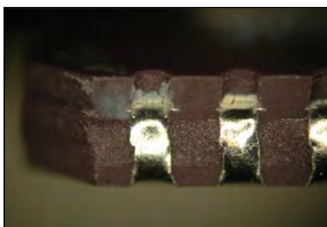
Figure 2. White residue in LCC castellations.
